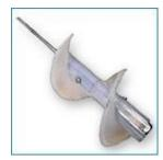
**Phoscrete Mixing Paddles**: The reverse corkscrew design allows fast mixing of Phoscrete HC, F1-HC and F3-HC kits in a standard 5-gallon bucket [**large mixer = 95 points**], or Phoscrete HC, F1-HC, F3-VO, and Primer in smaller quantities. [**small mixer =85 points**]. The auger action pushes the dry material down to the bottom of the bucket without splashing or overflow. The mixing paddle cleans-up easily with water.
