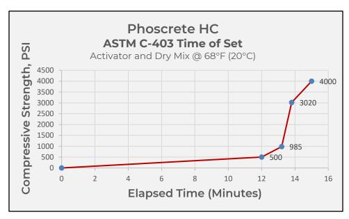
For ambient temperatures below 50°F (10°C), use the appropriate number of provided scoops of Phoscrete Fast-Set Admix to speed up the working time, in accordance with the charts on page [6] of this document.
