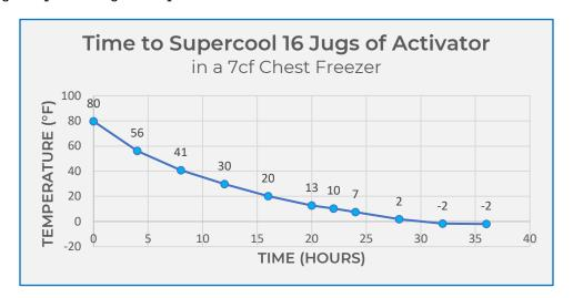
For concrete repair projects that require more than 16 kits of Phoscrete (7.5cf coverage), consider purchasing a larger chest freezer. A 15cf chest freezer will supercool 48 jugs of Phoscrete Liquid Activator from 85°F (30°C) to 10°F (-12°C) in less than [36] hours. Again, plan ahead when supercooling.
