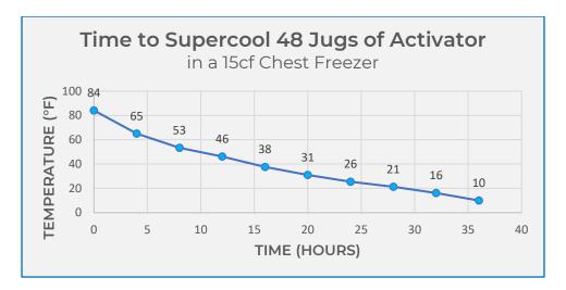
Just prior to driving to the jobsite, transfer 12-16 supercooled Liquid Activator jugs to a large cooler and cover with 40 lbs. ice. The temperature of the Liquid Activator is expected to increase on average 3°F per hour for the first [7] hours in the field. Then the temperature increases just 1°F per hour for the next [6] hours. Even in warm temperatures (85°F), supercooled Liquid Activator retains a cool temperature under 40°F (5°C) for longer than [24] hours without need to refresh the ice.
