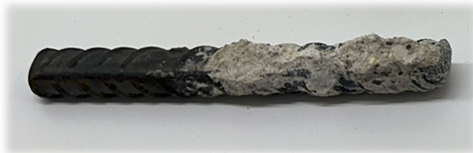
Figure 8 Phoscrete Rebar Coat (RC) applied to corroded rebar, bonds to steel and halts corrosion
