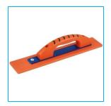
**Phoscrete Orange Thunder Trowel:** Phoscrete recommends Kraft Tools' polymer concrete float for the best finish because Phoscrete concrete formulas do not stick to plastics. [56 points]
